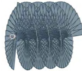
Fig. 1 Helix Filter segment: A multi spoke frame is used as a skeleton to hold the FabGuard material in a disk-like shape. The design provides two (2) open channels or pathways through the filter to reduce clogging.
