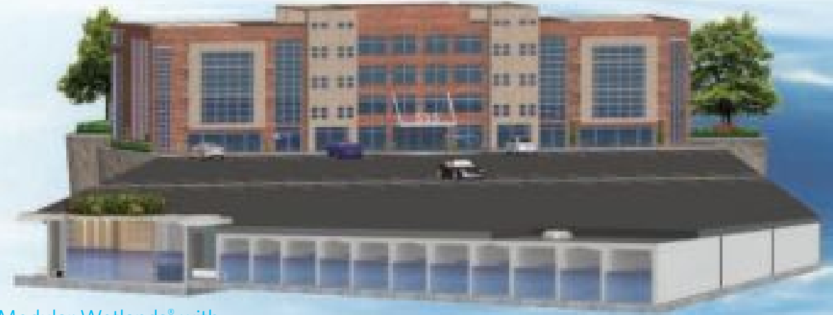
Modular Wetlands® with Box Culvert Prestorage
