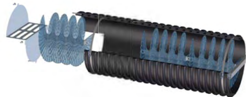
Fig. 2 A complete Helix Filter column consists of 3 or more Helix Filter segments inserted horizontally into a smooth lined plastic corrugated pipe. Each Helix Filter column will treat approximately 2.5 CFS.
