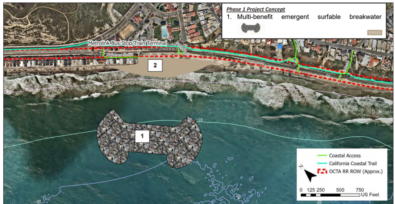
Figure 3-1: Conceptual Schematic for North Beach Multi-Benefit Emergent Breakwater
